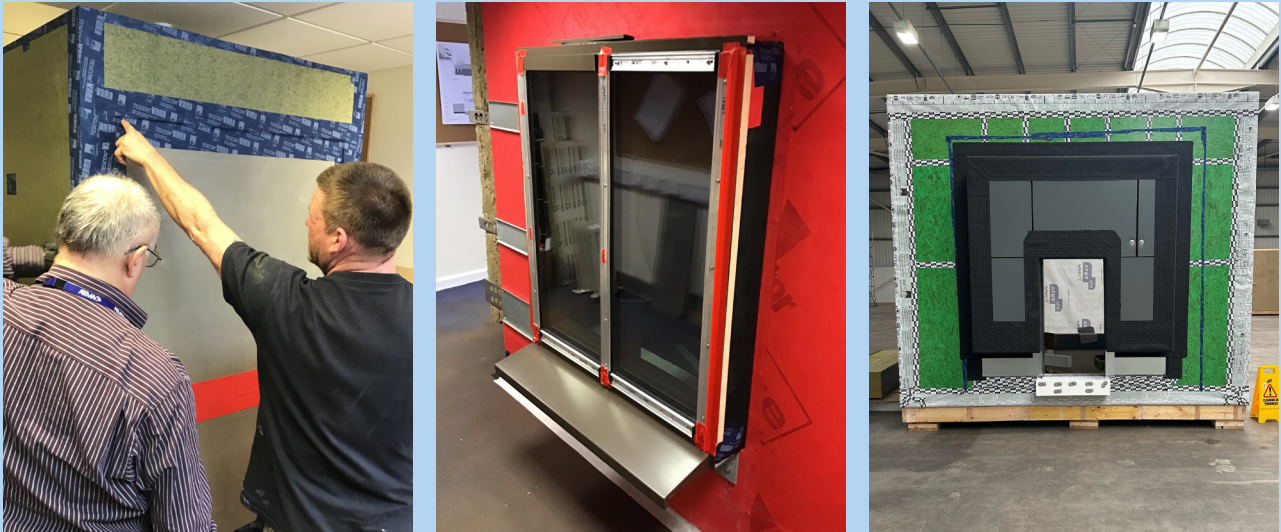
Fig. 26: From left to right: 1) The first TTARDIS (Testing, Training and Research rig for Design development, Installation & Sequencing) developed for the St Sidwell's Point project. 2) Example site mock-up, St Sidwell's Point. 3) Evolution of the TTARDIS. Image credits: Stephen Booth, Kier Construction & BE-ST.
