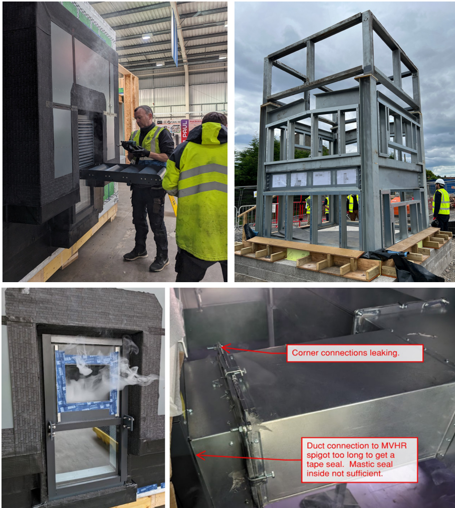
Fig. 12: Top left: BE-ST tardis test rig air testing. Top right: Faifley Campus test rig. Bottom: Component mock-up testing the installation and duct connections of an MVHR unit. Image credits: Morrison Construction
